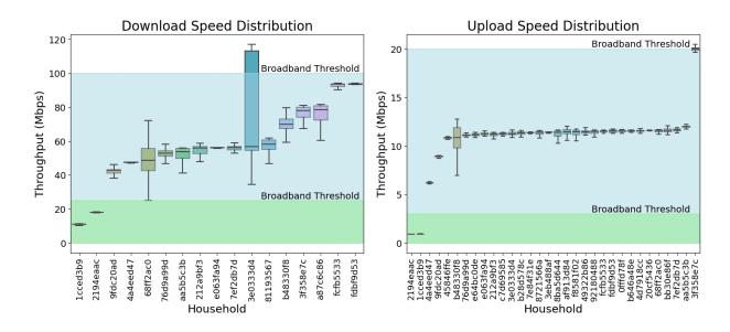
The boxplots of download and upload speed distributions for the Milwaukee devices identify 32 households, about 58% of tested households, without adequate broadband access (median throughput under 100 Mbps for download and 20 Mbps for upload).
